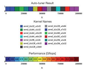
Figure 7. Result of auto-tuning for the SNRM2 kernel on a  $1 \times 16$  grid for vector sizes up to n = 1000000. Top; best kernel designated by color and name. Bottom; performance in Gflops/s.
