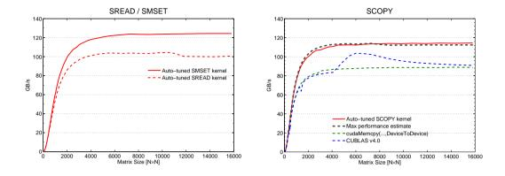
Figure 1. Left; the read (SREAD) and write (SMSET, i.e., memory set) effective bandwidth measured in GB/s using auto-tuned kernels for different size square matrices. Right; the measured performance and estimated maximum performance of the level 1 BLAS routine SCOPY using an auto-tuned kernel together with the performance of equivalent calls to cudaMemcpy (..., DeviceToDevice) and CUBLAS 4.0.
