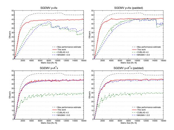
Figure 10. Performance of the auto-tuned SGEMV kernel (with TRANS = 'N' and 'T') on a Nvidia Tesla C2050 card. The curves show the average performance from ten calls.
