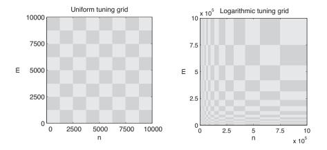
Figure 6. Tuning grids used by the auto-tuner for selecting the best parameters and kernels for different input matrix sizes  $m \times n$ . The left panel shows a uniform grid and the right panel a logarithmically spaced grid.
