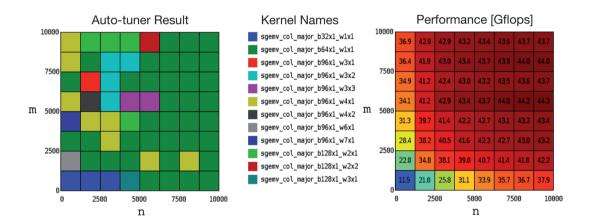
Figure 9. Result of auto-tuning for the SGEMV kernel on a  $8 \times 8$  grid for matrix sizes  $m \times n$  up to  $10000 \times 10000$  Left; best kernel designated by color. Right; performance in Gflops/s.
