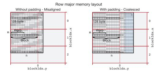
Figure 4. Access pattern for the row-wise reading of matrices having row major memory layout. Left; the misaligned case of arbitrary number of columns. Right; the coalesced case occurring when the number of columns is padded to a multiple of the warp size.
