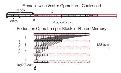
Figure 2. Coalesced access pattern for the element-wise operation on a vector and the subsequent parallel reduction operation per block in shared memory.
