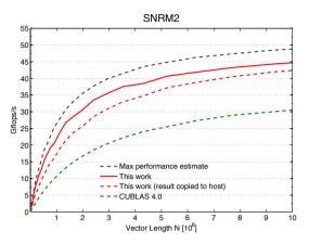
Figure 8. Performance of the auto-tuned SNRM2 kernel on a Nvidia Tesla C2050 card. The curves show the average performance from ten subsequent calls to the kernel.
