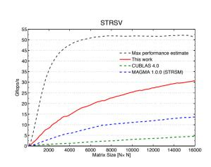
Figure 12. Performance of the auto-tuned STRSV kernel on a Nvidia Tesla C2050 card. The curves show the average performance from ten subsequent calls to the kernel.
